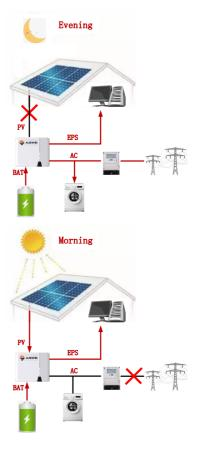
normal conditions, the battery does not discharge, only in the event of GRID failure as a backup power supply to the load.
